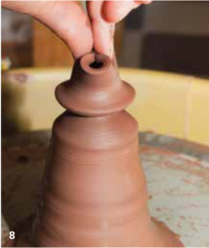
8 Pinch the slightly flared rim of the knob together in the middle, leaving two openings on each end.
