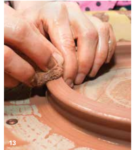
13 Throw a bottomless ring on the wheel. Compress it while slowly pulling the ring outward to create a wall for a tray.
